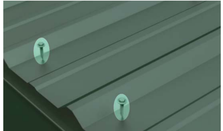
Figure 55. Attaching Roof Panel to Wood Decking
